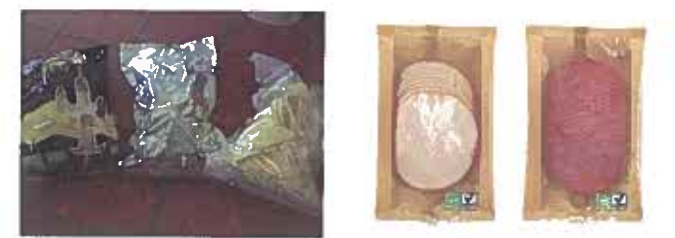
Figure 1b. Tortillachips packed in reference (l) - natureflex type 2 (m) - Natureflex type 1 (r)
